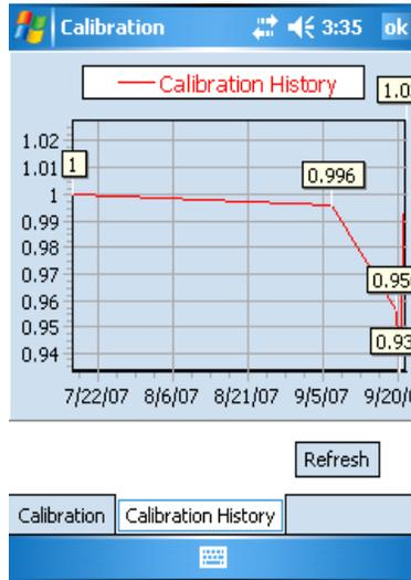
Diver-Pocket is also capable of reading and displaying the calibration history from CTD-Divers. Each time a CTD-Diver is calibrated, the settings are saved to the CTD-Diver's internal memory. This feature is useful for monitoring changes in calibration over time which may aid in explaining significant variations or anomalies in data.
